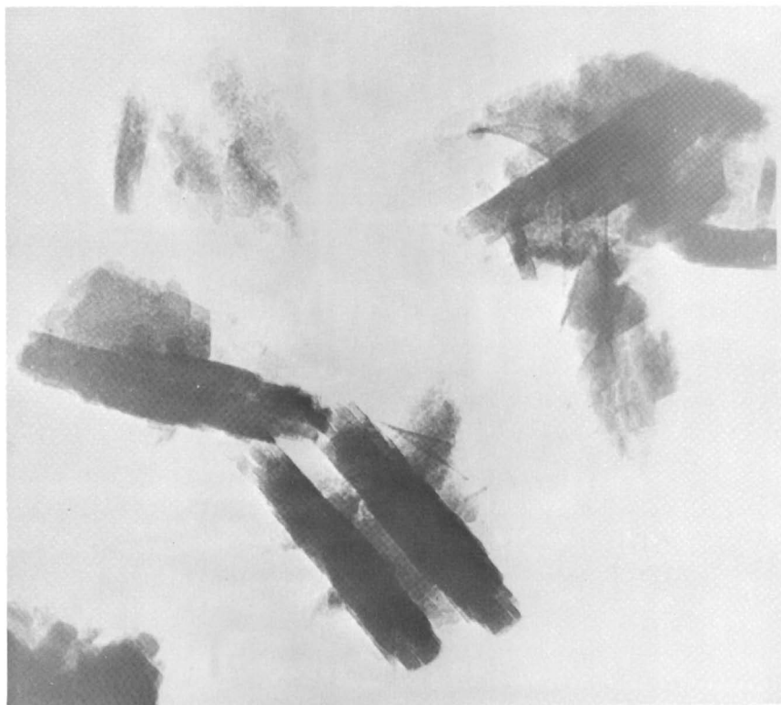
Figure 9. Electron micrograph of a carbon replica of ZSM-3 (CSZ 168), magnification 83,520 \times
