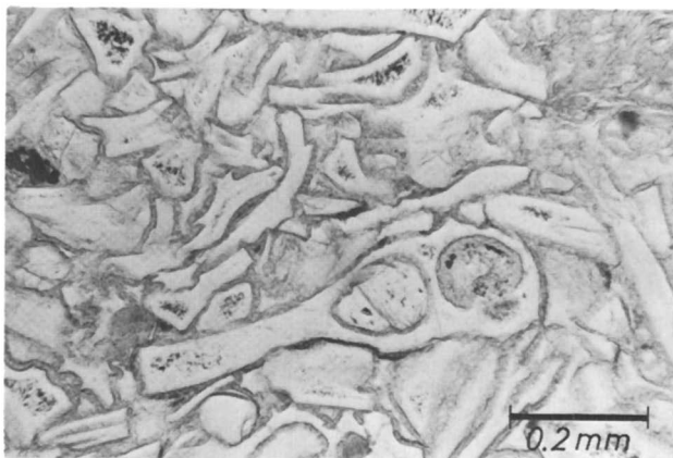
Figure 1. Microscopic photograph of zeolitized Nakanosawa rhyolitic vitric tuff. Clinoptilolite replaces glass shards and fills vesicles within the glass.
